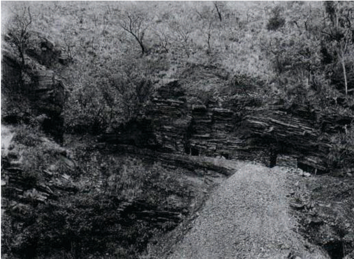
Crocidolite workings in gently inclined banded ironstone: Leather's Mine (Pietersburg Asbestos Ltd) east of the Malips River
